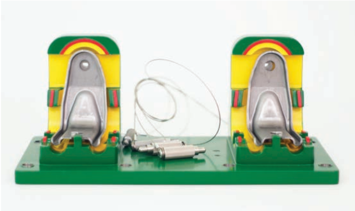
Early iteration of the check fixture
